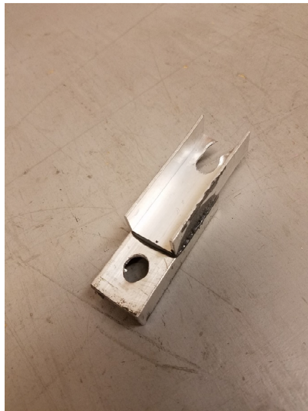
Figure 4. Aluminum to aluminum bonded with JB Weld, showing connection tear-out
